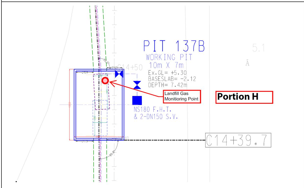
**Figure 4.5 Monitoring Location – Pit 137B (137 Pit B)**
